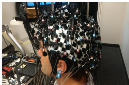
**Figure 1.** Configuration of emitters and detectors producing 105 acquisition channels. Channel locations are determined with a Polhemus Patriot 3D digitizer based on the standard 10-20 system.
