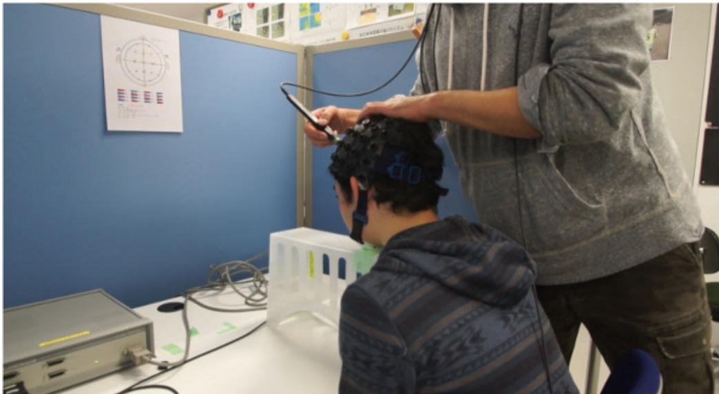
**Figure 5: Calibration of optode position.** A magnetic digitizing tool was used to determine placement of 10-20 landmarks on the head and position of the optode channels. [Please click here to view a larger version of this figure.](#)
